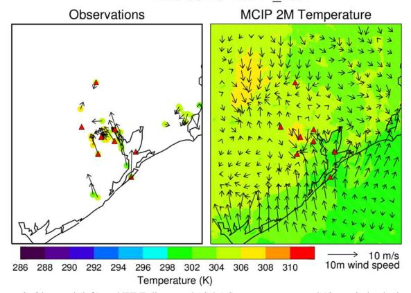
Figure 2. Observed (left) and WRF diagnosed (right) 2 m temperature and 10 m wind velocity at 23 UTC 25 September 2013 from the new 1 km WRF simulation. Strength of WRF simulated bay and sea breezes are in better agreement than in the original simulation (Figure 1).
